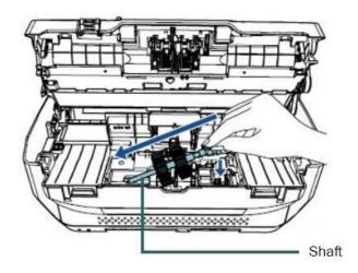
b. Rotate the bushing on the pick shaft in the direction of the arrow below
