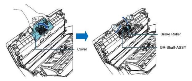
4. Remove the brake roller from the Brake Roller Shaft Assembly
