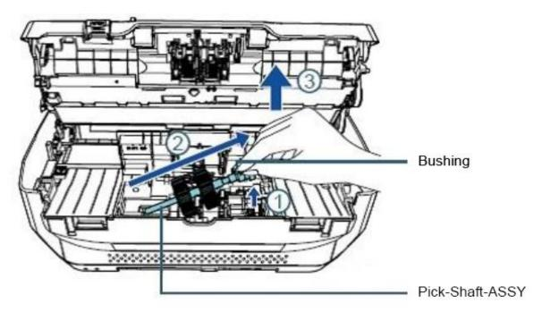
\*Be careful not to touch the gear near the bushing on the shaft as it contains grease\*
